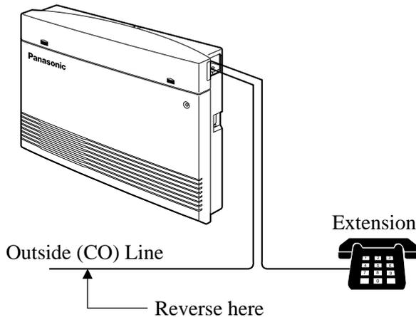
1. Complete all the required extension wiring.
