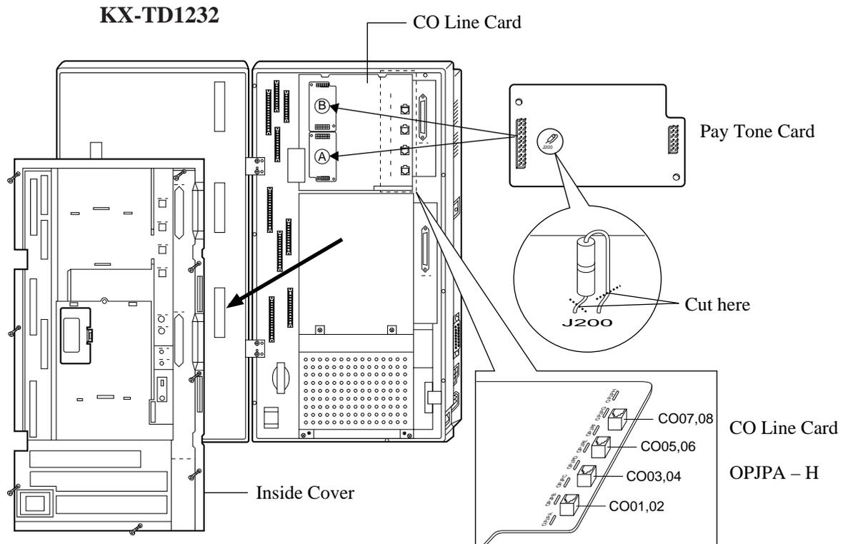
3. If you do not cut the wire of the J200 in Pay Tone Card, the detected mode is 16 KHz. If you cut the wire of the J200 in Pay Tone Card (Open Mode), the detected mode is 12 KHz.
