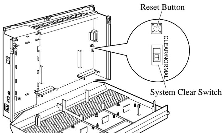
**CAUTION** • Before touching the System Clear Switch and Reset Button, put on a grounding strap.
