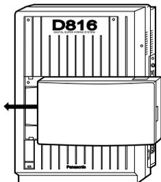
**Installing the DISA Card (KX-TD199) to the Remote Unit (KX-TD198) /
