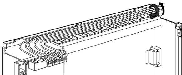
4. To remove the rivet, use a screw driver as shown below.
