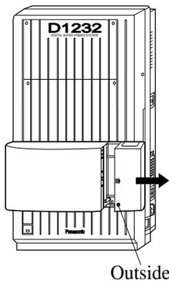
5. Secure the inside screw (included) to fix the cabinet to the main unit.
