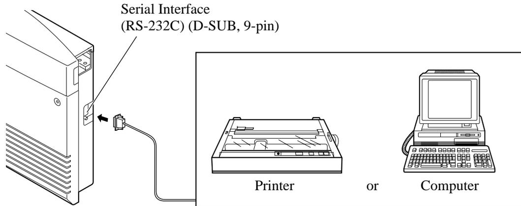
Arrange the cables so that the printer will be connected to the system as shown in the appropriate chart on the following page.
