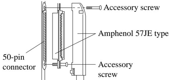
2. To attach the Amphenol 57JE type (Plug) to the connector, drive the accessory screw into the upper part.
