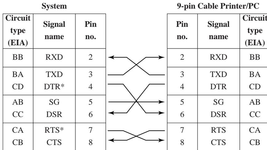
If you connect a printer or a PC with a 25-pin cable, follow the chart below.
