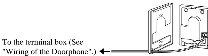
4. Secure both halves together and re-install the screw.
