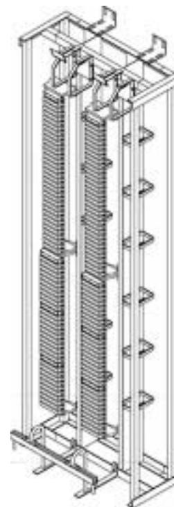
Main Distribution Frame HVt-COM-B2-2 for LSA-PROFIL®-2/10 (System) and 2/8 (Lines)
