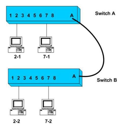
Looking at the diagram above ports 1 through 4 are assigned to VLAN1 and ports 5 through 8 are assigned to VLAN3 on each switch. The switches are interconnected over an ISL trunk link. Which of the following actions would test proper VLAN and trunk operation? (Choose three.)
