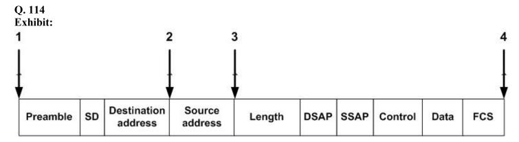
Catalyst Switches have three primary operating modes that are used to handle frame switching Cutthrough, Store-and-forward and Fragment-free looking a the frame shown in the diagram which point is the store-and-forward switching decision made?
