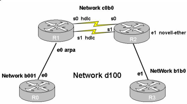
You want to create a sub interface on serial 0 on Router R2. Which of the following is the correct syntax to create this sub interface 2?
