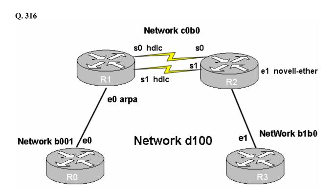
You are configuring R2 so that it can communicate with R1 on serial port s0. What encapsulation should you use on s0 to setup this IPX network?
