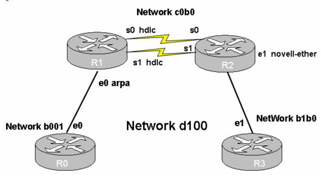
You are configuring R3 so that it can communicate with R2 on Ethernet port e1. What encapsulation should you use on s0 to setup this IPX network?
