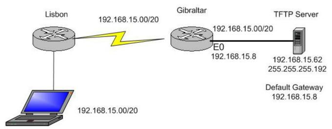
A network administrator has installed a new router in the Lisbon office and is unable to backup the IOS image of the new router to a TFTP server located in the Gibraltar office. Given the network diagram, identify the source of the problem.
