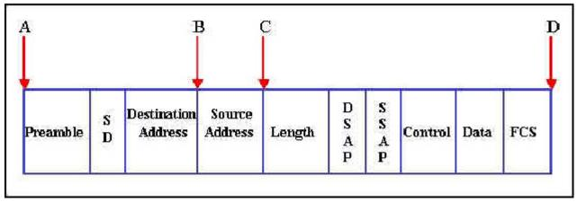
At what point in the frame shown in the diagram is the store-and-forward switching decision made?
