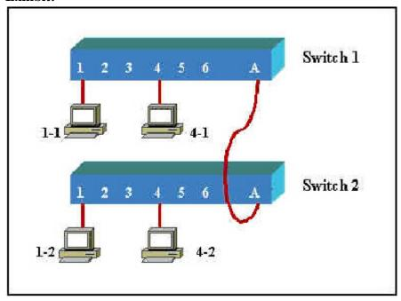
Given the network diagram, assume that ports 1 through 3 are assigned to VLAN1 and ports 4 through 6 are assigned to VLAN2 on each switch. The switches are interconnected over a trunked link. Which of the following conditions would verify proper VLAN and trunk operation? (Choose three.)
