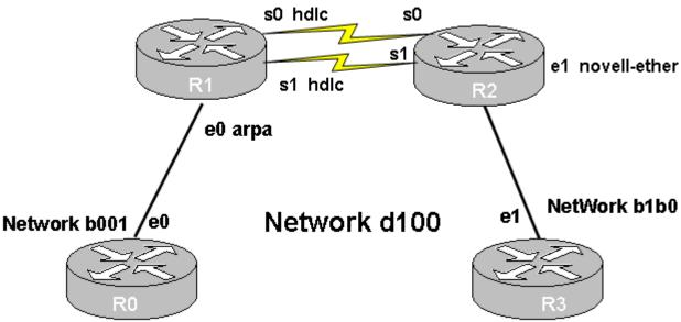
Which encapsulation type should be used for the e1 port of Router R3?
