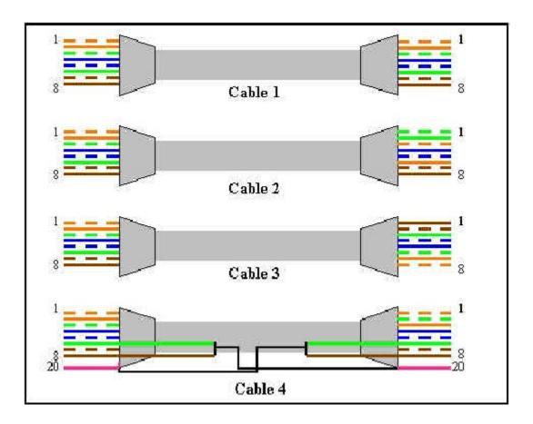
Choose the correct cable to connect an Ethernet switch to another Ethernet switch.
