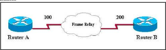
Which Frame Relay feature allows the point-to-point Frame Relay PVC between Router A and Router B to be identified at Router A as 100 and at Router B as 200?
