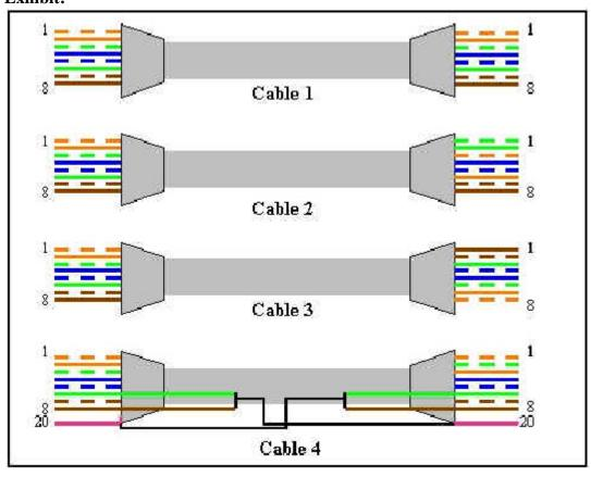
Choose the correct cable to directly connect a router to another router over the Ethernet.
