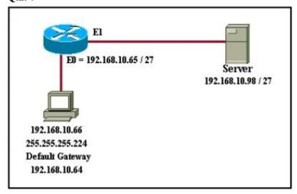
Company ABC has just added an employee workstation to its network. The employee is unable to connect to the server at IP address 192.168.10.98/27. Identify the incorrectly configured network parameter.
