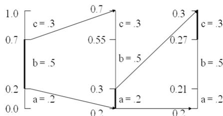
**Fig. 1.** Example of arithmetic encoding of the input sequence 'bac'. Symbols of the alphabet  $A = a, b, c$  have probabilities of occurrence  $P = .2, .5, .3$  Final range is  $[0.27, 0.3)$ . The sequence 'bac' can be thus coded with 0.27.
