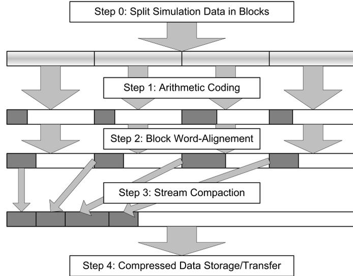
**Fig. 2.** Block-Parallel GPGPU Simulation Data Compression Process
